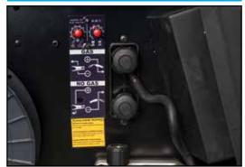
Easily change the electrode polarity for use with solid wire (electrode positive) or flux core wire (electrode negative).
